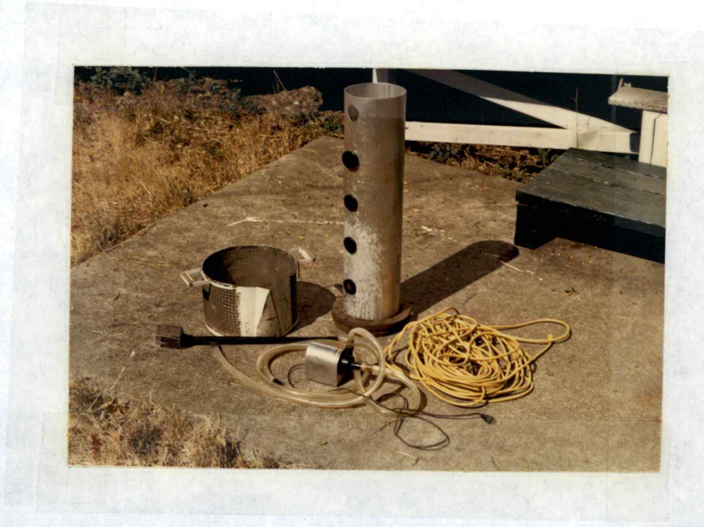
Figure 3. Gorman-Rupp centrifugal pump sampler.
