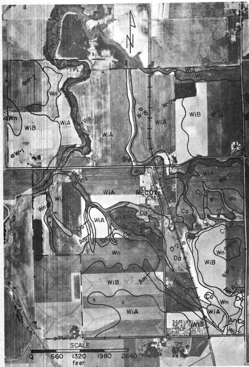
Figure 10. Soil map of the McCoy study area. Sample sites, major roads, and railroad are shown. Am = Amity silt loam; Co = Concord silt loam; Da = Dayton silt loam; Wa = Wapato silt loam; WiA = Willamette silt loam, 0 to 3 percent slopes; WiB = Willamette silt loam, 3 to 12 percent slopes; Wn = Woodburn silt loam soils.
