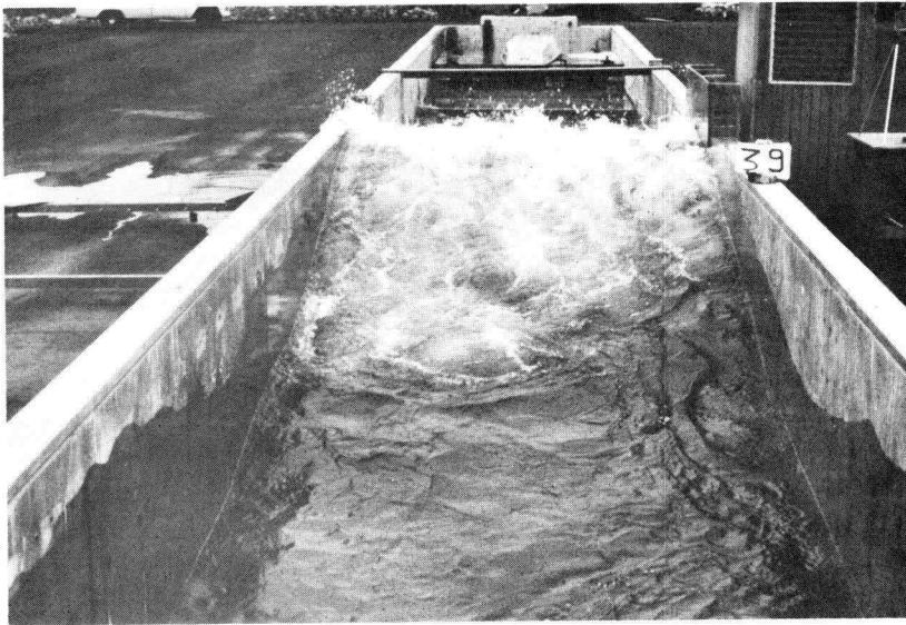
Fig. A-15. Non-Breaking Overtopping, 1:10 Scale Model
