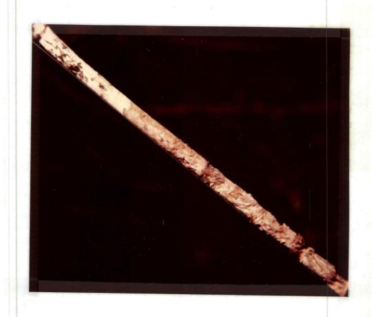
Figure 3. A core extracted by increment borer exhibiting stain and decay caused by Phellinus weirii.
