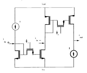
Fig. 2.10. Half-Delay and Full-Delay Realization in SI Circuits.
