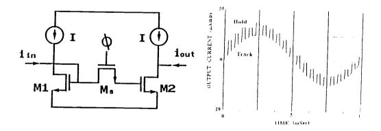
Fig. 2.15. Clock feedthrough in a track-and-hold circuit and SPICE results.
