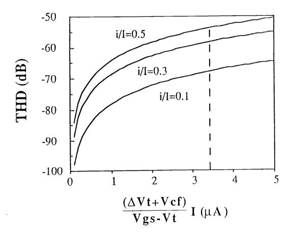
Fig. 2.19. Total harmonic distortion due to the clock-feedthrough and mismatches.
