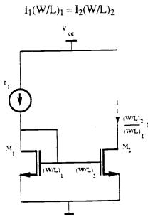
Fig. 2.4. Simple Current Mirror.
