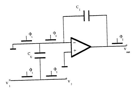
Fig. 2.12. A parasitic-insensitive differential input SC integrator.
