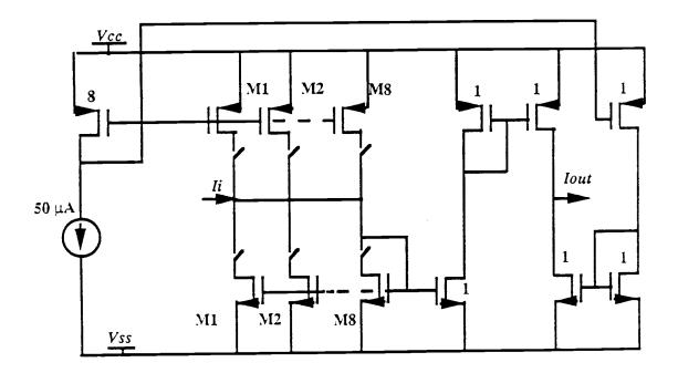
Fig. 4.3. Center Frequency Programming Block.
