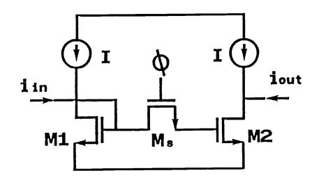
Fig. 2.18. Clock Feedthrough in a Track-and-Hold Circuit.
