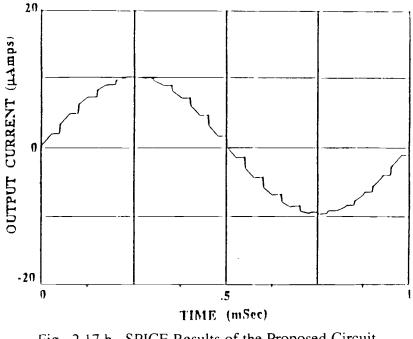
Fig. 2.17.b. SPICE Results of the Proposed Circuit.
