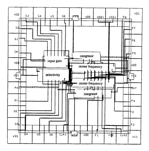
Fig. 4.8. Main blocks of the circuit and the chip layout.
