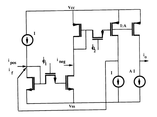
Fig. 2.11. Differential input-switched current integrator with scaled outputs.
