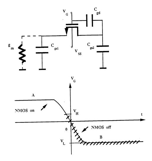
Fig. 2.14. Clock Feedthrough.
