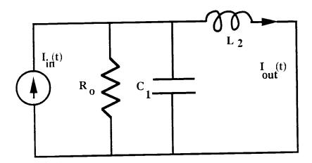
Fig. 3.1. A Singly-Terminated RLC Second-Order Lowpass Filter.
