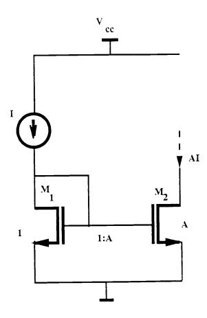
Fig. 2.6. Scaling in a Simple Current Mirror.
