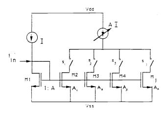
Fig. 2.7. A Current Amplifier with Scaled Mirroring Transistors.
