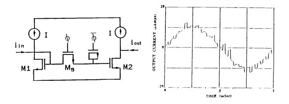
Fig. 2.16. Suggested Circuits for Clock Feedthrough Cancellation with Dummy Switches and SPICE results.
