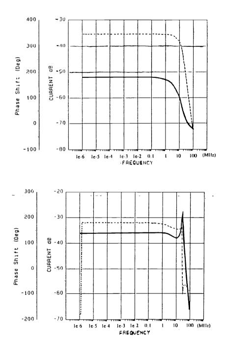
Fig. 4.7. Simulations of Frequency Responses of a Current Amplifier with the Source Follower.
