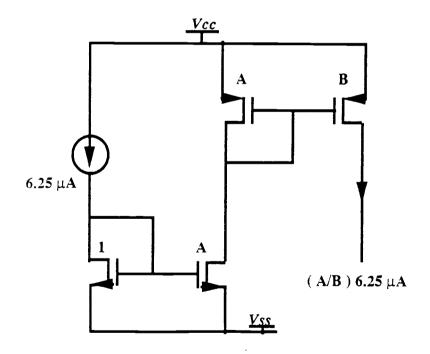
Fig. 4.5. Current Carrying Before Mirroring.
