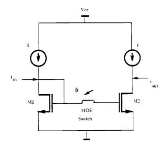
Fig. 2.8. Tracking Mode in an SI Circuit.
