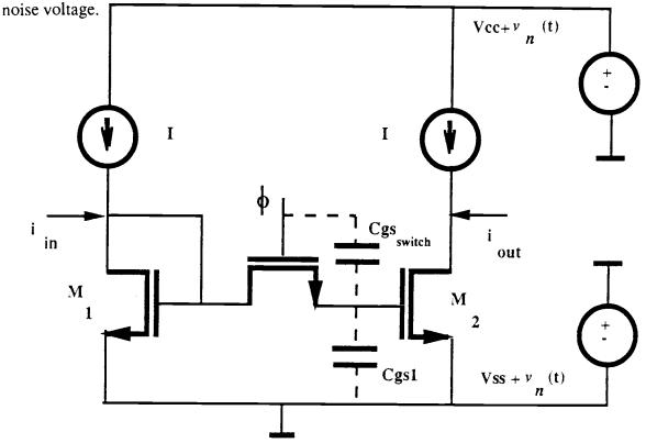
Fig. 2.3. Simple Current Mirror with the Noisy Power Supplies.
