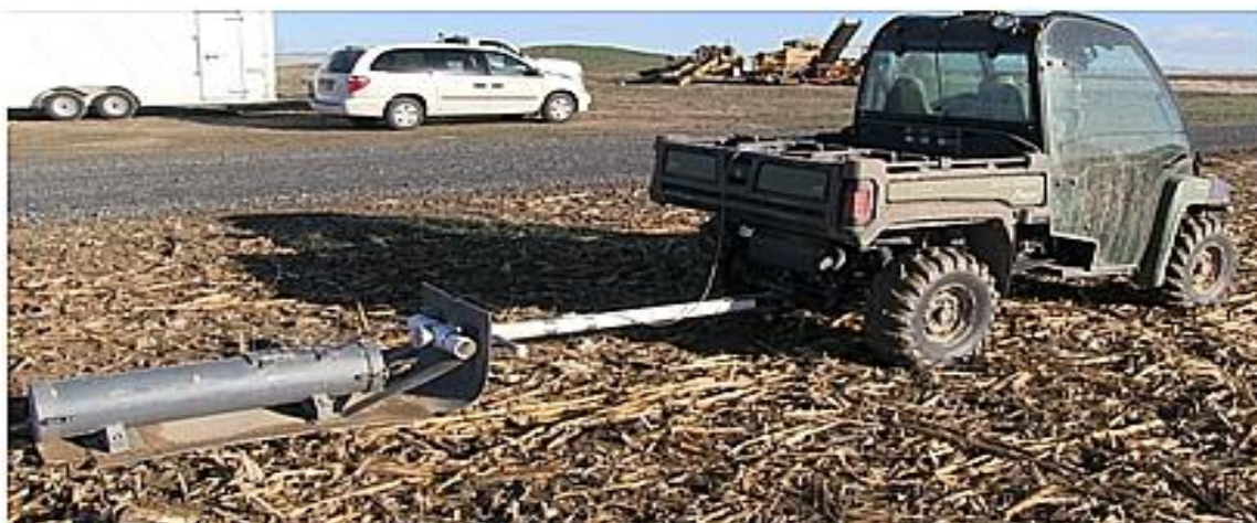
Figure 3-3: Geonics EM38 and towing assembly
