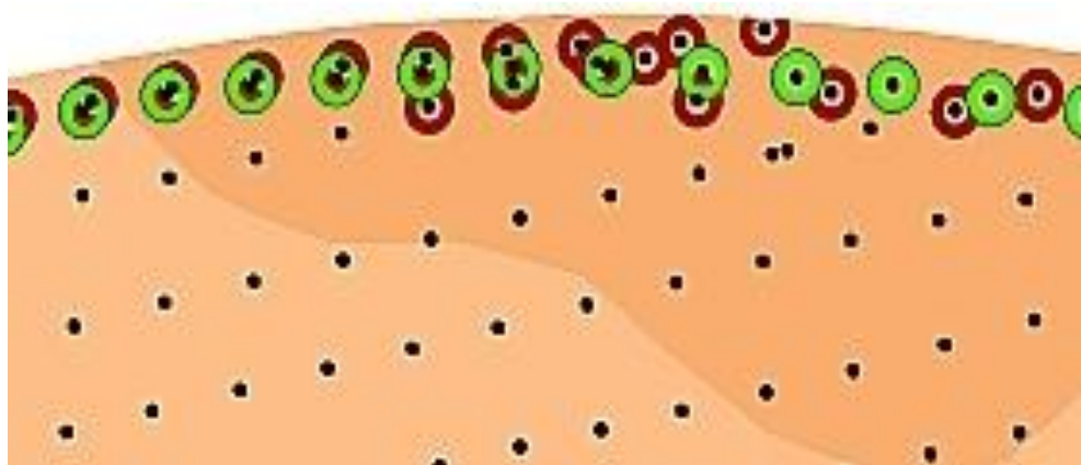
Figure 3-9: Map of EM38 samples used for consistency checks Edge points used for consistency checks circled: green indicates control points (contiguous measurements); red indicates test points.
