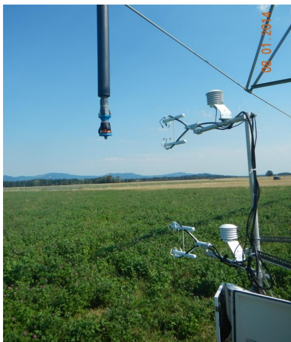
Figure 5-8: IRGASON instruments at two heights, August 2014
