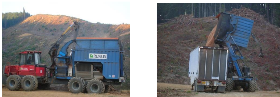
Figure 1.2 Mobile chipper processing forest residues near Elkton, Oregon , USA. Processing a road-side pile (left); unloading a bin of chips into a set-out trailer.
