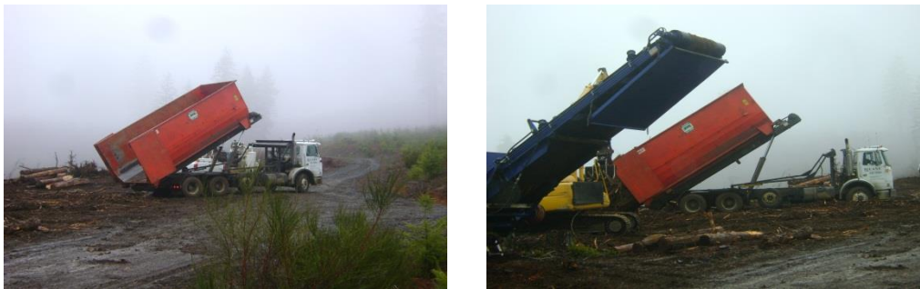
Figure 1.4 Hook-lift trucks in biomass recovery operations near Eugene, Oregon, USA. The trucks were transporting residues to a centralized landing where a stationary grinder was located.
