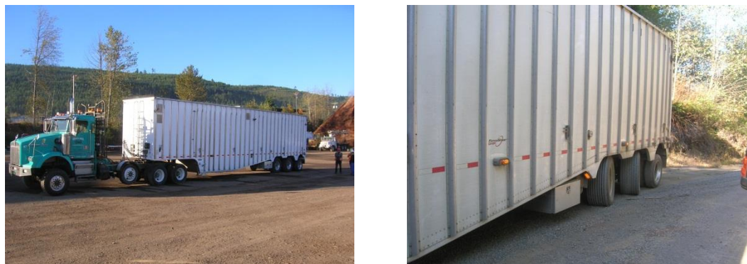
Figure 1.7 Rear-steer axle chip trailer operating in Port Angeles, Washington. This configuration is comprised of a tri-axle trailer (left) with two steering axles (right).
