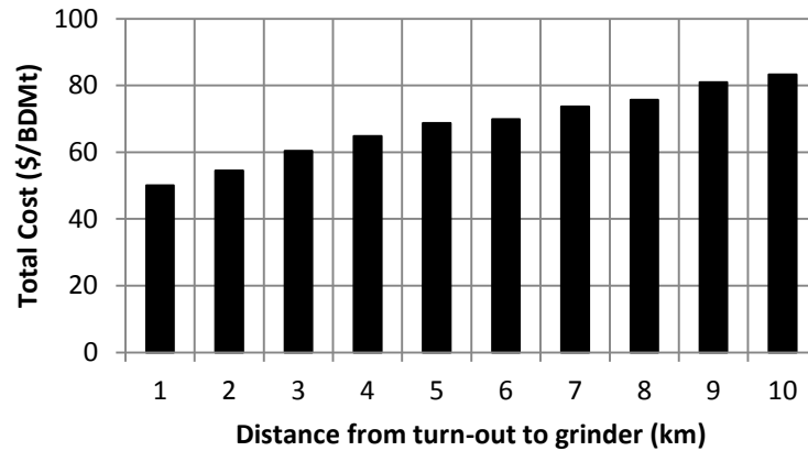
Figure 3.9 Sensitivity of total cost to changes in truck turn-out-grinder distance, study site Case I.
