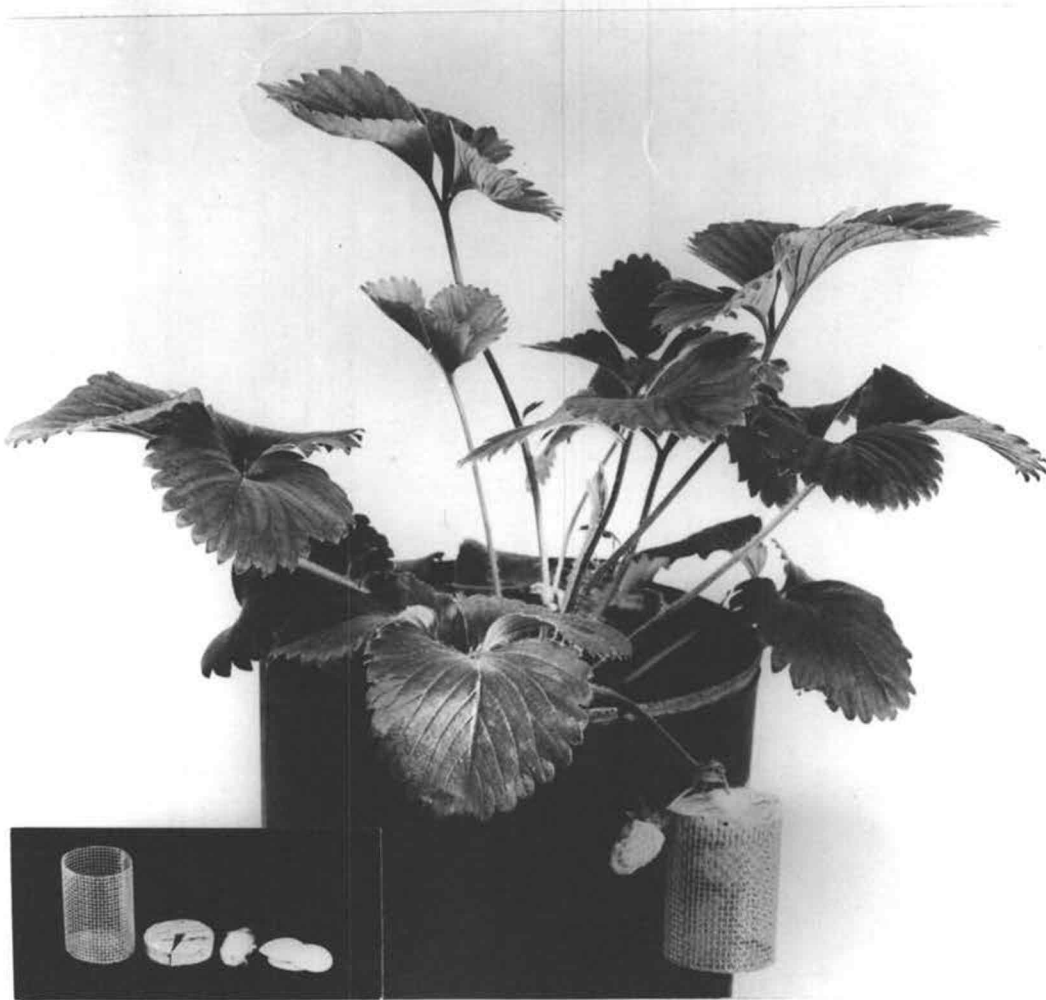
Figure 1. Individual moisture chamber used in greenhouse pathogenicity experiments. Insert (lower left) shows chamber made from plastic-coated window screening, cork with petiole insertion slit, cotton for plugging slit and absorbent paper discs for producing high humidity in chamber.
