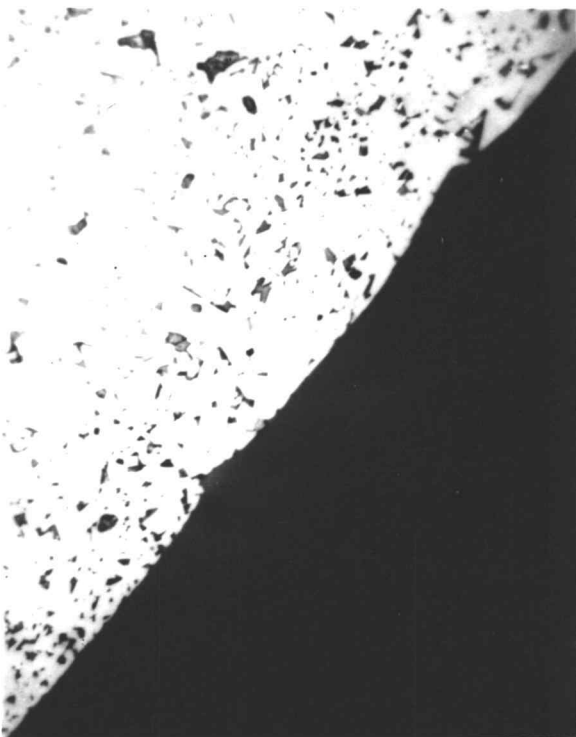
Figure 12. Al 2 O 3 seal heated at 1100°C for 8 hrs. and furnace-cooled. 500X.
