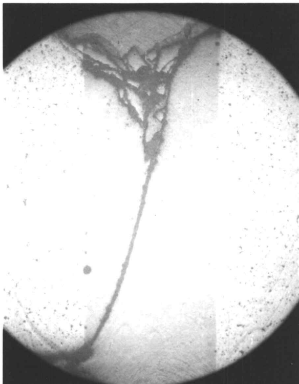
Figure 28. Cross-section of \text{Al}_2\text{O}_3 seal formed at 900^\circ\text{C} . 25X.
