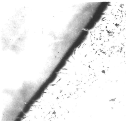
Figure 20. F66 seal held at 1200°C for 5 sec. and furnace-cooled. 250X.
