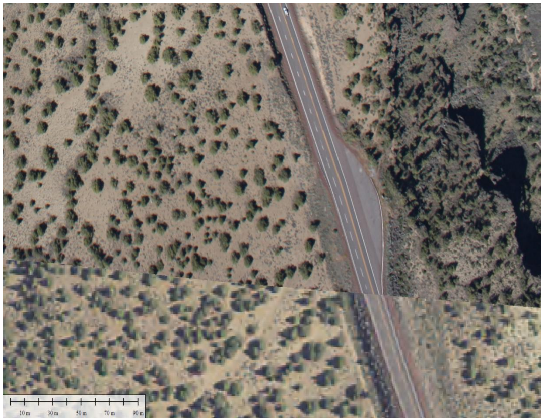
Figure 3.13: Displacement error when using aerial Image Positioning Tool because of image rotation and/or crabbing of the Aircraft.
