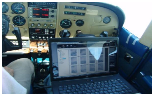
Figure 3.5: A laptop computer is mounted in the Cessna 182 aircraft and connected to the 12.40 megapixel Canon EOS Rebel XSi and GPS to collect aerial images every 5 seconds, storing the data in a 1.5 terabyte external hard drive.
