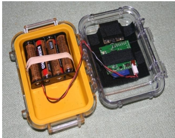
Figure 3.6: The self-contained WAAS GPS device used on our study. Approximately 98.90% positions of a sample of 38,600 positions taken during a static test (open sky, 2m above level ground) were within 5 m of the true location. Mean error was 1.76m (Std. Dev. 1.08m) and the maximum error was 12.2m over 38,600 continuously logged points (10.72 hours).
