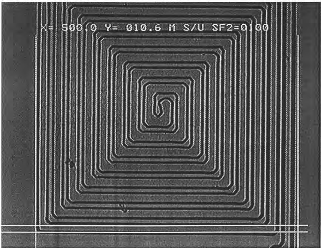
Figure 4.1: Photoresist pattern of the first lithography layer of a square capture dot with 10\ \mu\text{m} lines and 10\ \mu\text{m} spacing between electroplated lines.
