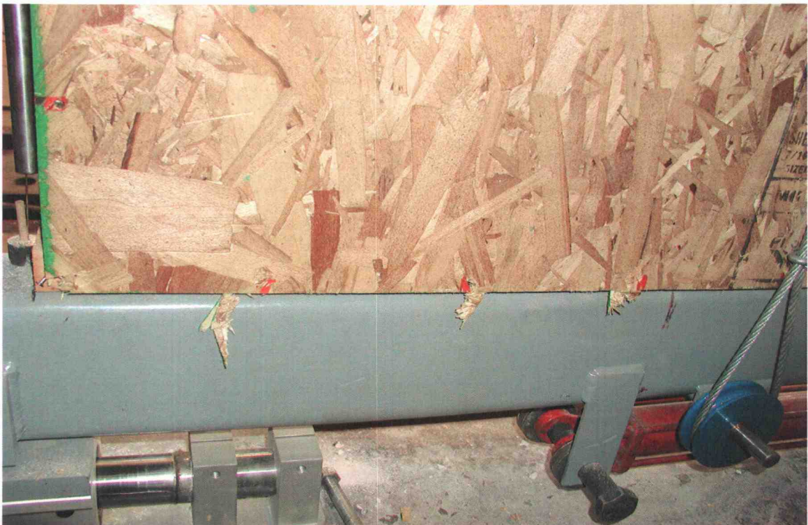
Figure 23. OSB sheathing edge breakout along the sill plate
