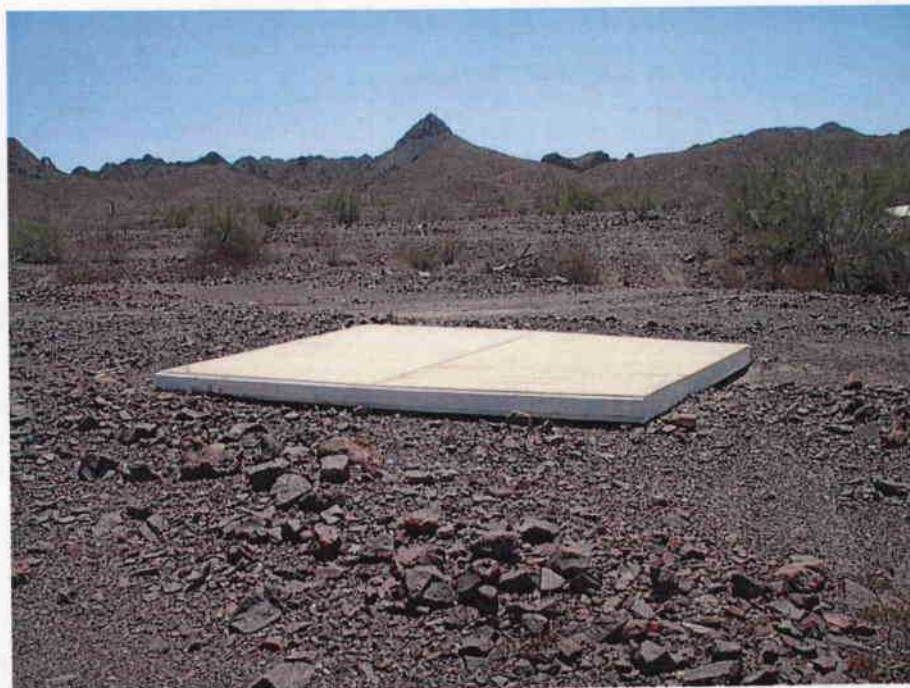
Figure 49. Ground photograph of the alluvial fan in Yuma Wash, Arizona. In the forefront is one of several calibration panels deployed for remote sensing studies.
