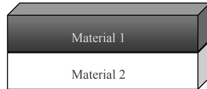
Composite with materials of different CTE's
