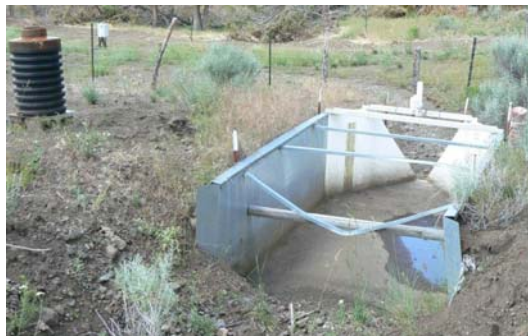
Mays flume 4 days after the same storm. Floor of flume has dusting of sediment but floor is already dry.
