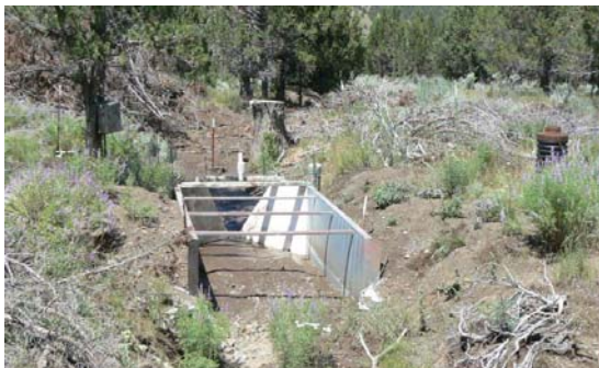
Jensen flume 4 days after summer thunderstorm, notice sediment deposits in the floor of the flume.
