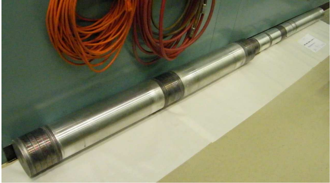
Figure 4-7: Internal components of PGNAA Collimator
