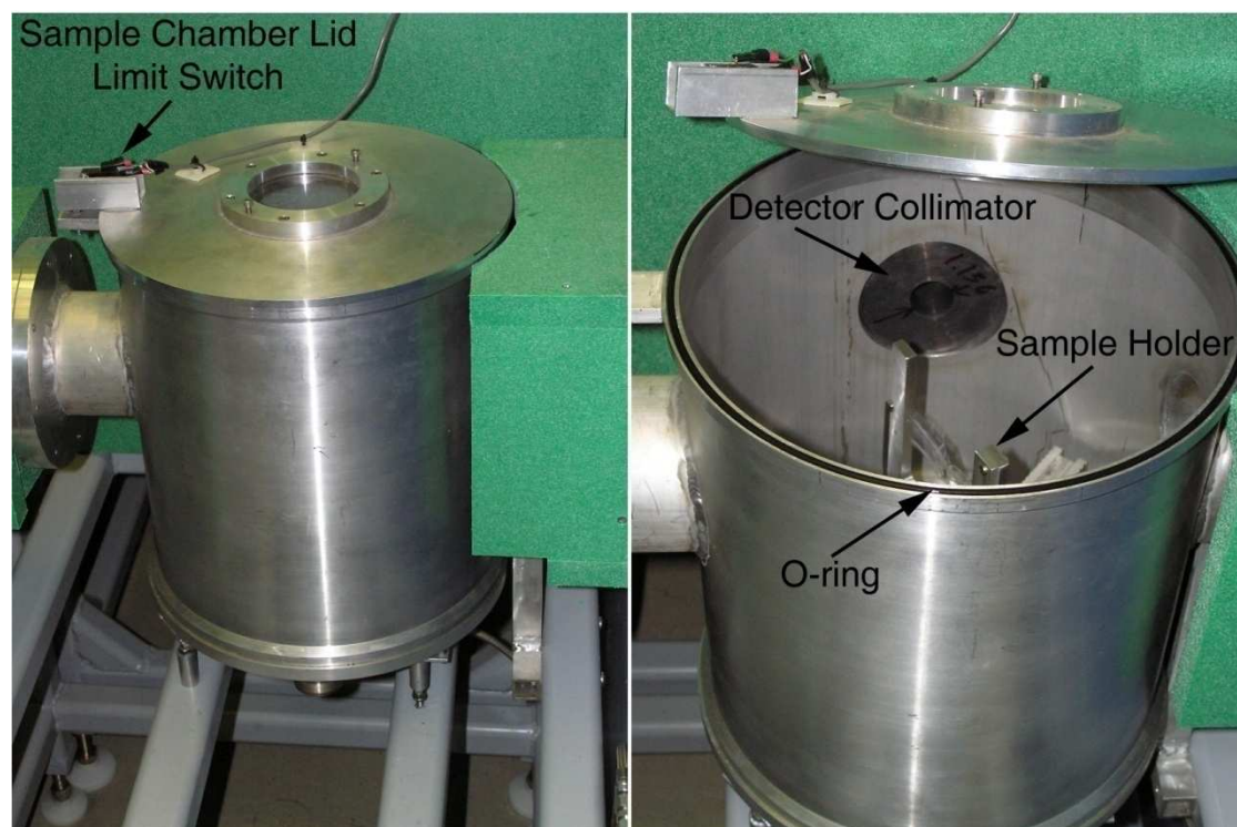
Figure 4-29: PGNAA Sample Chamber
