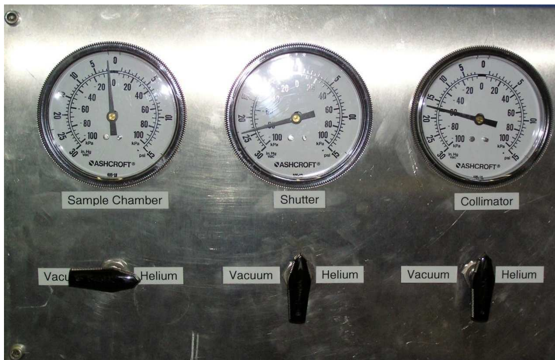
Figure 6-3: shutter evacuation and fill controls
