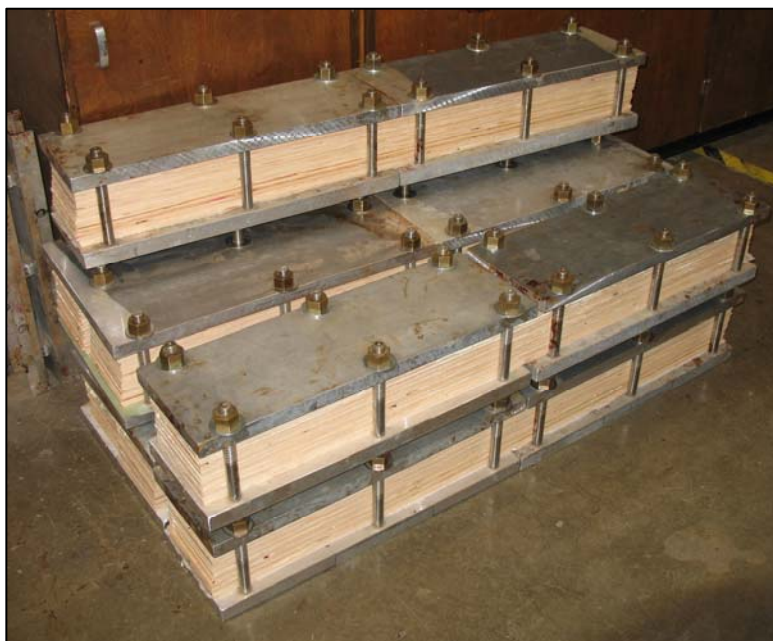
Figure 7.9. Cold pressed LVL specimens during manufacturing.
