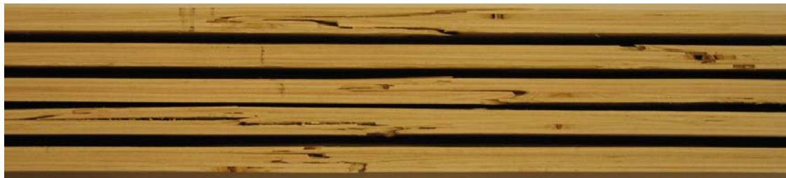
Figure 7.13. Typical LVL tension failures showing failure through layers.
