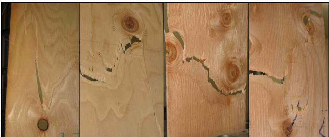
Figure 3.16. Specimen failure at knot and sloped growth ring pattern locations.
