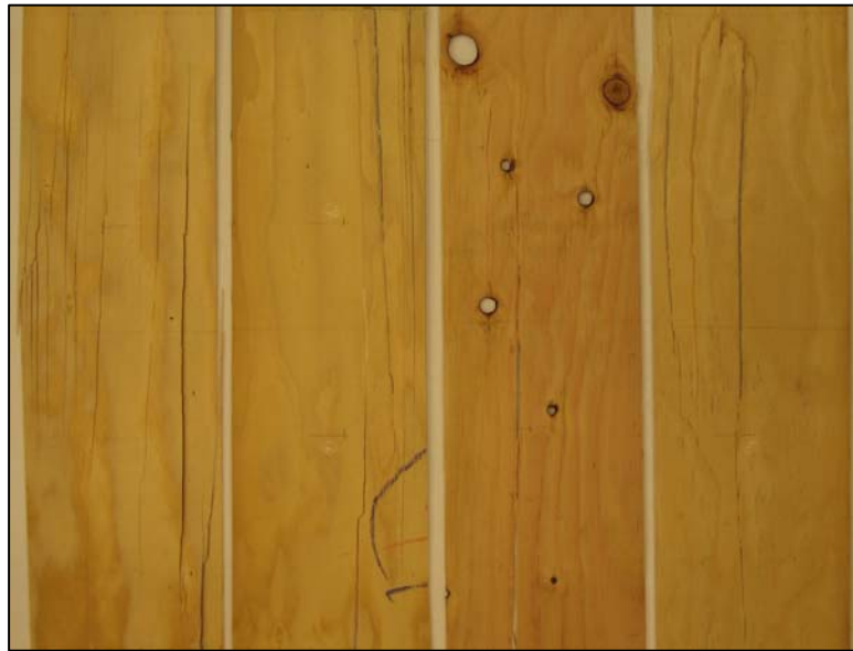
Figure 3.15. Failure when growth rings were oriented parallel to specimen length.
