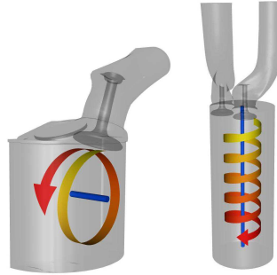
Figure 3.6: Idealized in-cylinder flow through a gas engine (left) and a diesel engine (right). Figures 1.1 and 2.1 show the visualization of CFD data simulating such flows.
