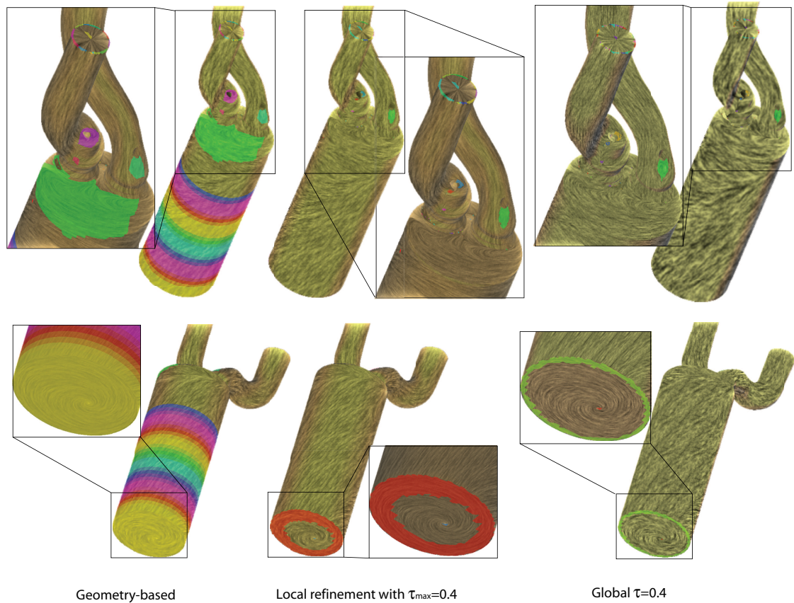
Figure 8.9: This figure shows the results of Morse decomposition before (left) and after automatic hierarchical refinement (right) for the diesel engine simulation dataset. The setting for the hierarchical refinement is r = 2 , \tau_{max} = 0.4 , and maximum number of iterations equal 60. The Morse sets are colored differently to emphasize their difference. Note that how the automatic framework produces the comparable results (middle) to the ones using a global \tau (right).
