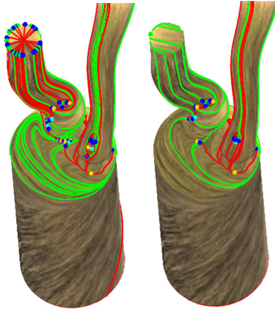
Figure 4.5: User-guided flow smoothing on CFD data simulating in-cylinder flow through a diesel engine: before (left) and after (right).
