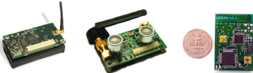
Figure 1.2: Examples of sensor nodes used in a wireless sensor network.
