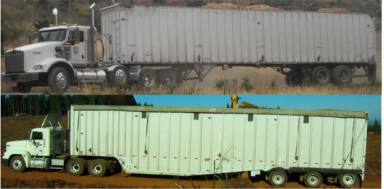
Figure 3.2. Chip Trucks used in the study. A tandem driving axle 20-foot tractor, drop axle in raised position, with a tandem axle 45 feet live floor chip van trailer (Top); and a tandem 18-foot tractor with a tri- axle 48-foot chip van trailer with a drop center (bottom).
