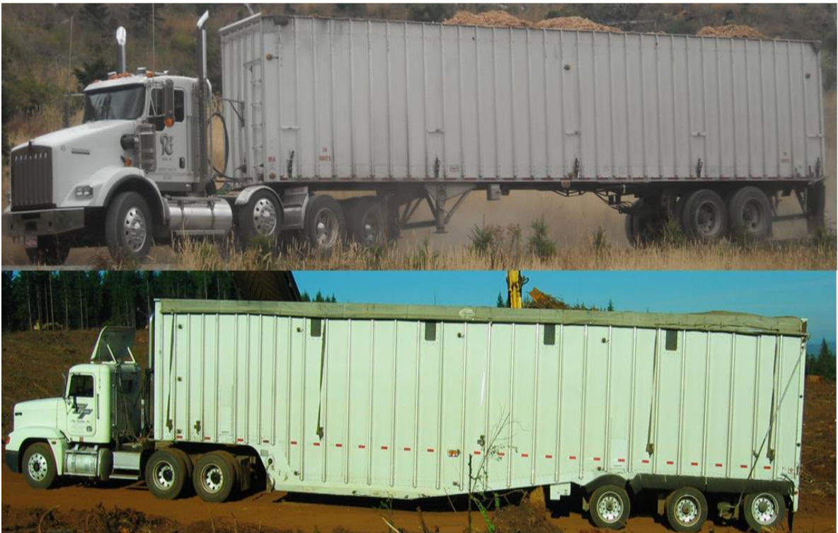
Figure 4.2. Chip trucks used in the study. A tandem driving axle 20-foot tractor, drop axle in raised position, with a tandem axle 45 feet live floor chip van trailer (top); and a tandem 18-foot tractor with a tri- axle 48-foot chip van trailer with a drop center (bottom).
