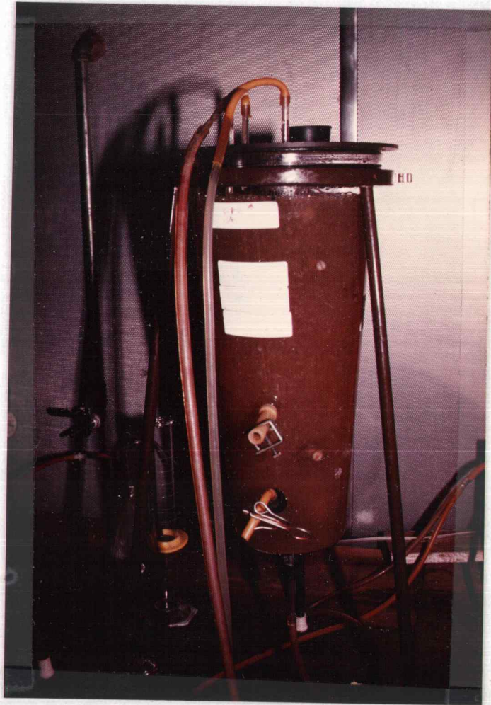
Apparatus used for Complete-Mix, Continuous Flow Reactor with Cell Recycle.
