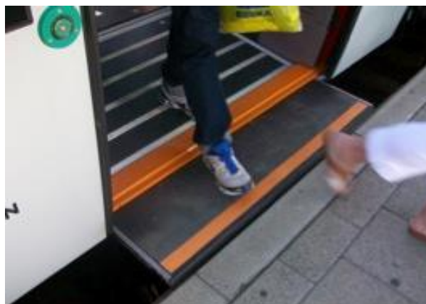
Figure 15: Automatic Gap Filler Shown on a German LRT
