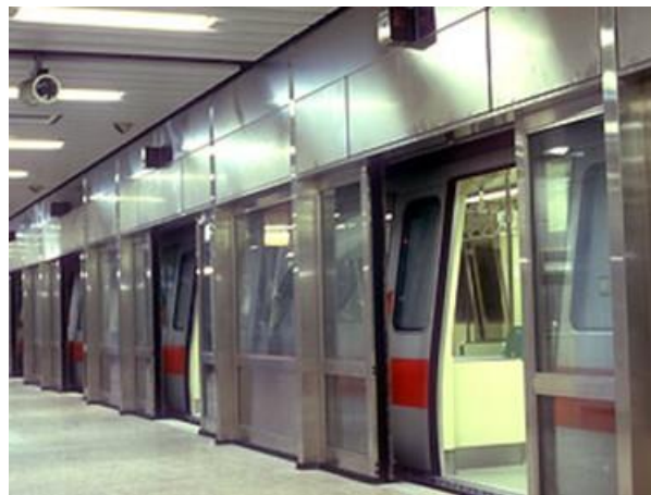
Figure 5: Full platform screen doors Paris (PB Bulletin)
