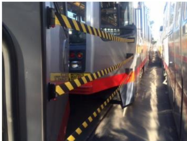
Figure 3: Elastic Band Between Car Barriers in San Francisco, CA.
