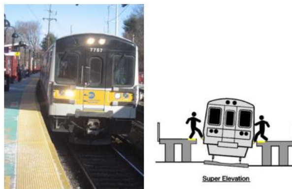
Figure 1: Superelevation in Relation to Gap (15)
