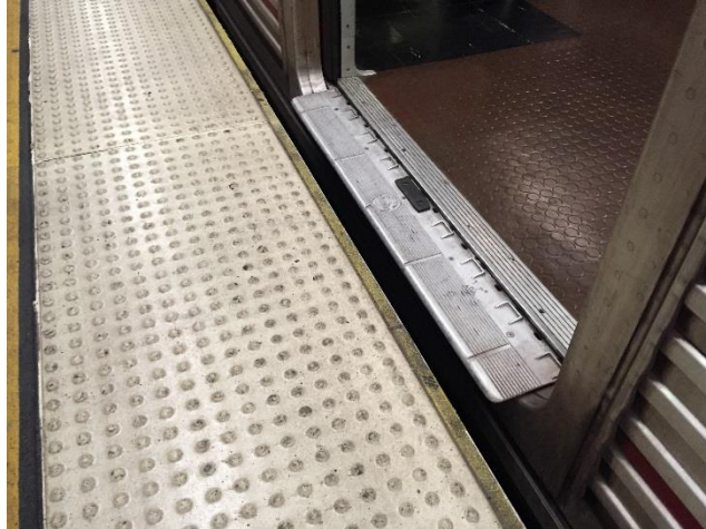
Figure 29: Extended Door Thresholds (LA Metro)
