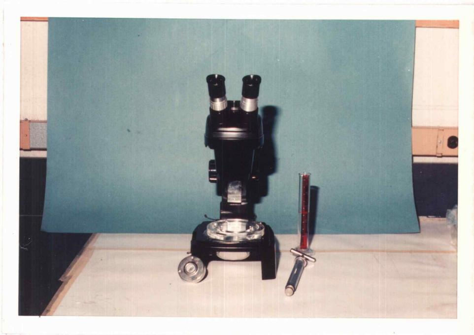
Figure 14. Counting apparatus. Center: Dissecting microscope with counting wheel on stage. Right foreground: Stempel pipette.
