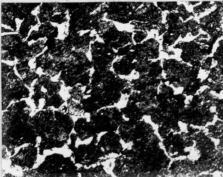
Fig. 10 Annealed 0.97% Carbon Steel, Electrolytic Polish 20 Seconds, 2% Nital Etch, 250X.
