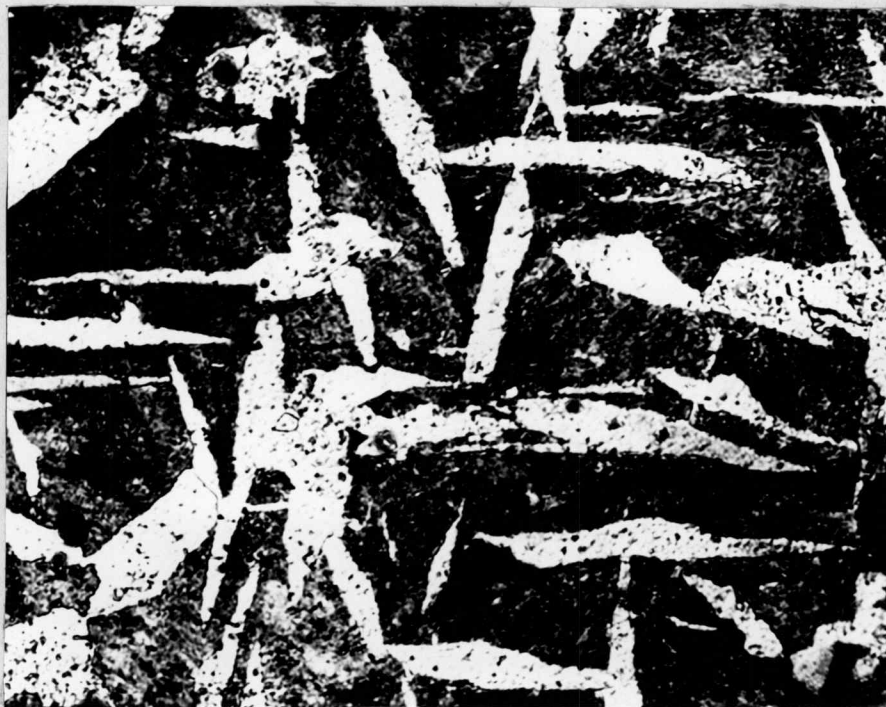
Fig. 12 Medium Carbon Cast Steel, Electrolytic Polish 30 Seconds, 2% Nital Etch, 250X.
