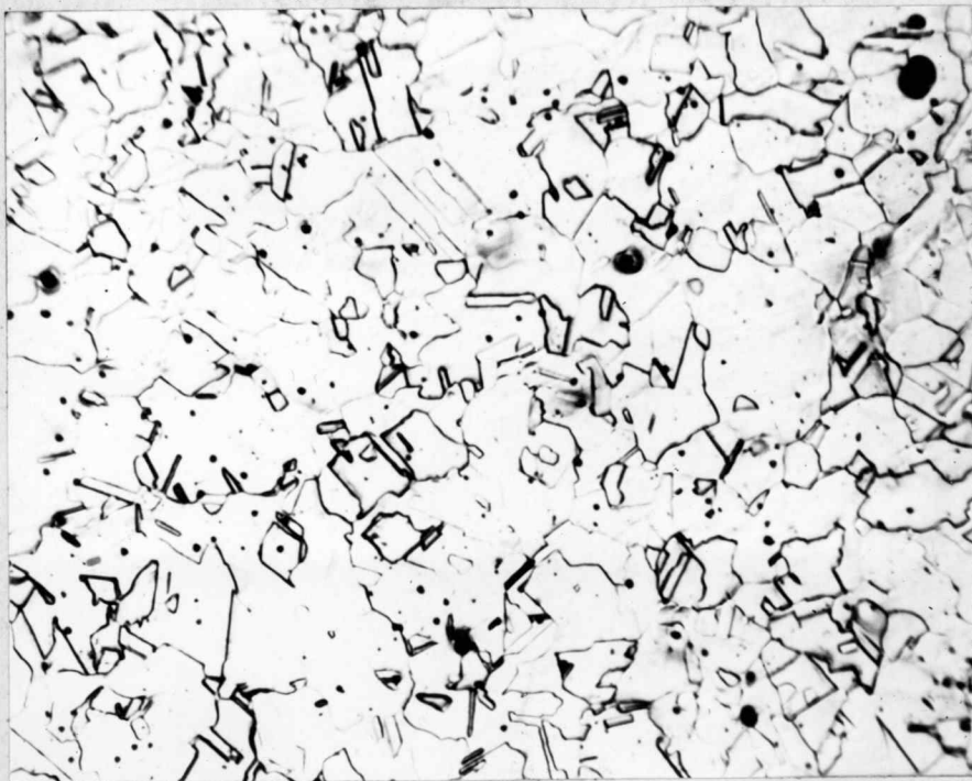
Fig. 21 Monel Metal, Electrolytic Polish 10 Seconds, \text{HNO}_3-\text{H.C}_2\text{H}_3\text{O}_2 Etch, 250X.
