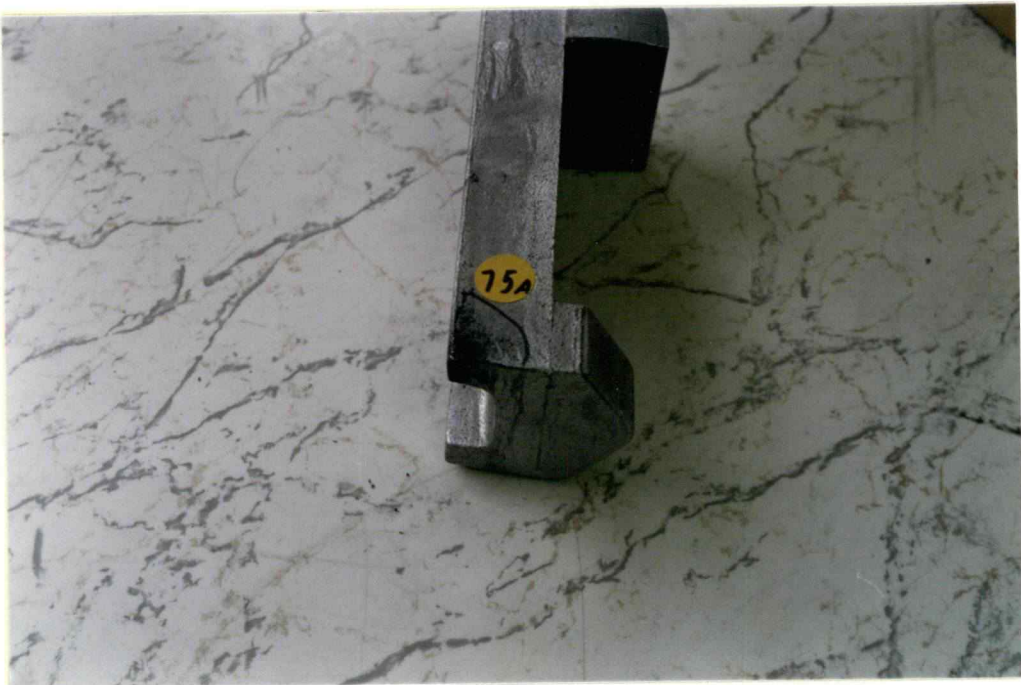
Figure 7: Example of Sand Penetration
