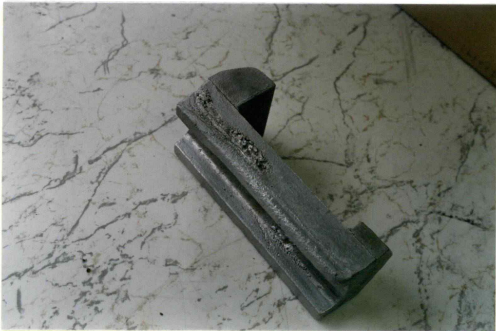
Figure 5: Example of Cuts and Washes
