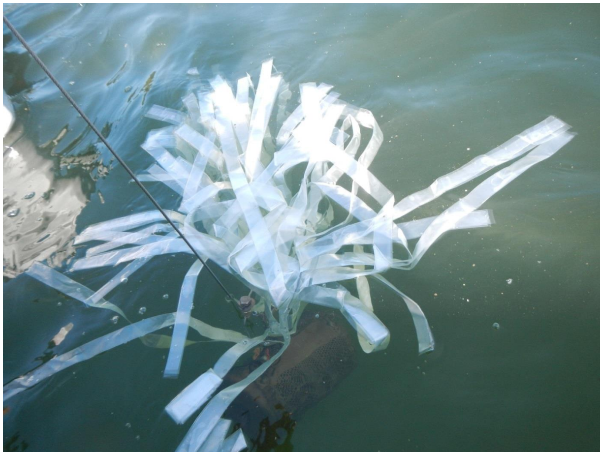
Figure B2. Deployment configuration of LDPE passive samplers as they were lowered into the river. PRC-containing LDPE were housed in a stainless steel cage, samplers for bioassays (no PRCs) were cage-free.
