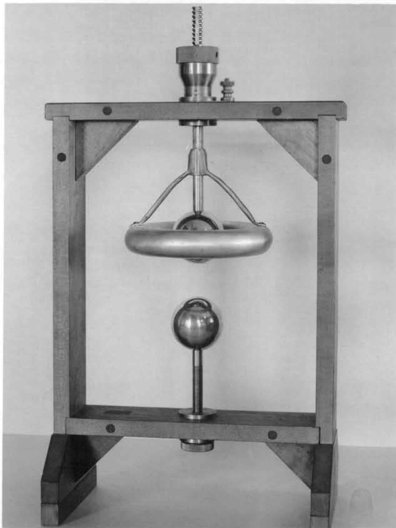
FIG.4 SHIELDED 6.25-cm. SPHERE-GAP, USING UPPER SHIELD ONLY.
