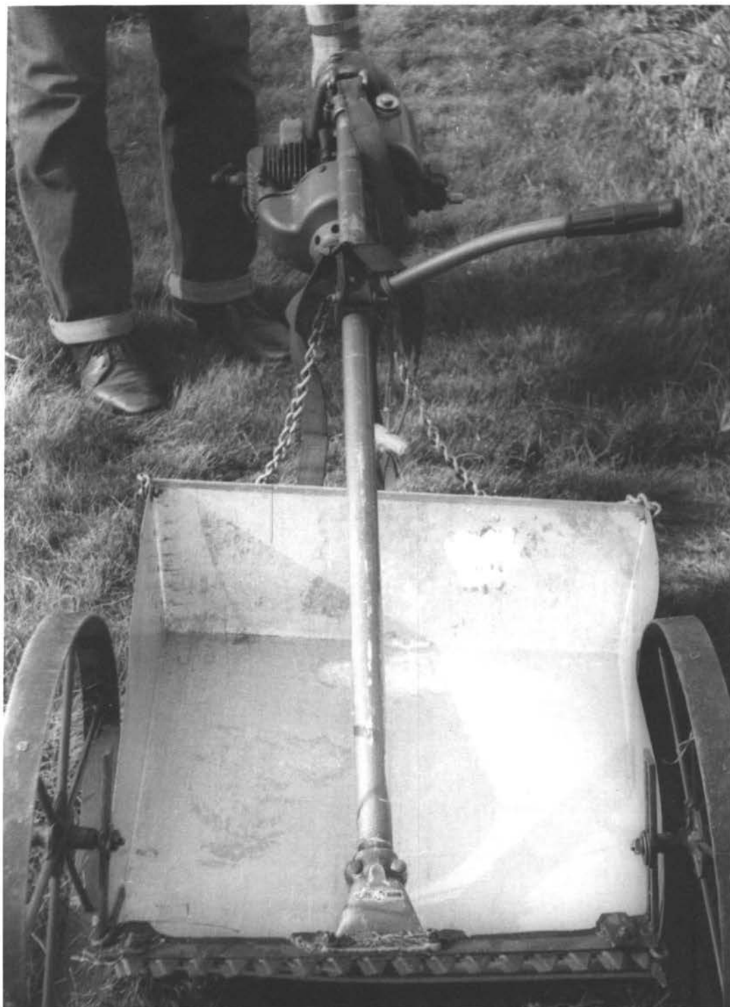
Figure 4. Front view of the Scythette mower used for clipping the plots. Note the forage catching pan and the manner in which the wheels are mounted to facilitate adjustment of the mower bar height.
