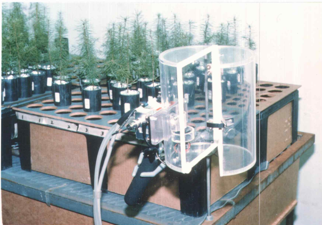
Figure 2. Photograph of the cuvette used in combination with the LI-6000 in these experiments.
