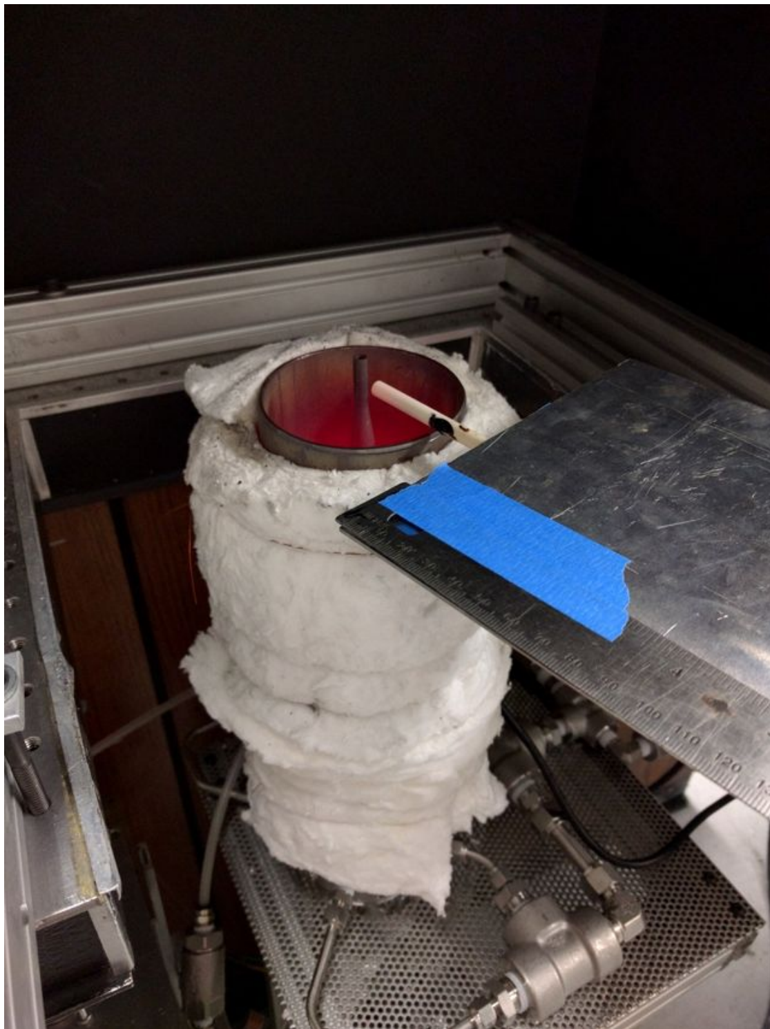
Figure 3.5: Photograph of coflow temperature distribution measurement setup
