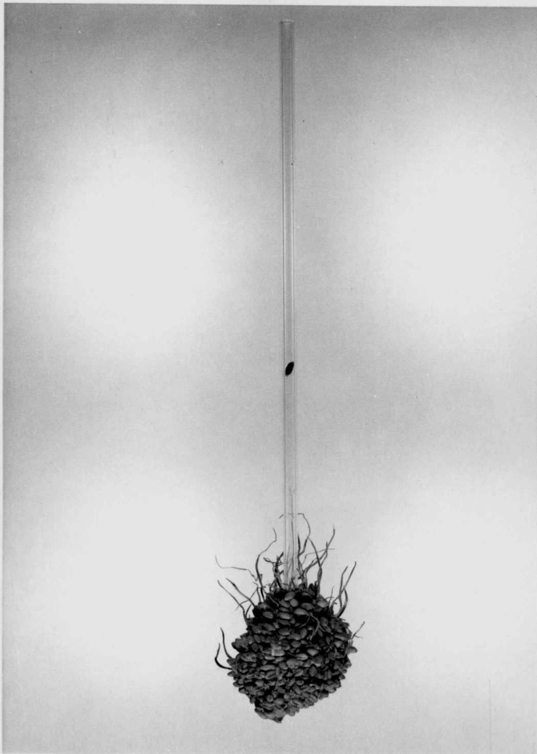
Figure 10. The ball of fungus infested grain from the center of laboratory Experiment Two, a fungus hot spot with no insects involved.
