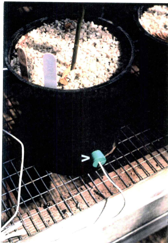
Figure 3-2. Photograph showing experiment pot set-up with soil thermocouple psychrometer in place.
