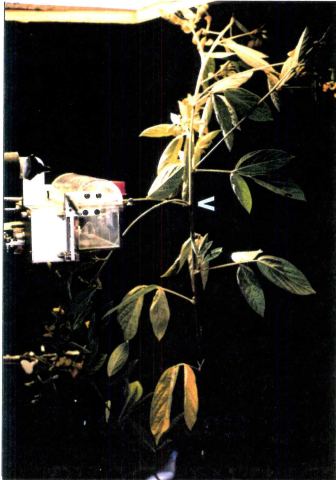
Figure 3-3. Photograph showing portable CO 2 infrared gas analyzer. Measured leaf is highlighted.
