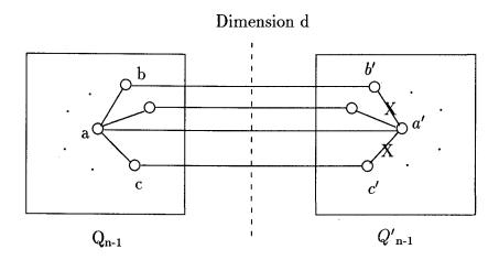
Figure 4.6. Case when all faulty links are incident to a single node. Here, node a' has two faulty links, (a', b') and (a', c'), incident to it.
