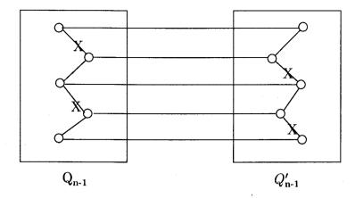
Figure 4.3. Faulty  $Q_n$  in which no node has more than one faulty link incident to it. Lines with X indicate faulty.
