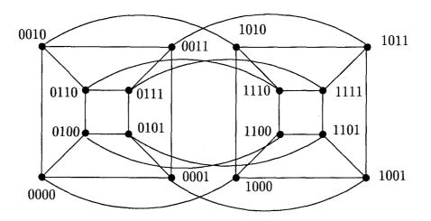
**Figure 1.1.** Construction of  $Q_4$  from two  $Q_3$ 's.
