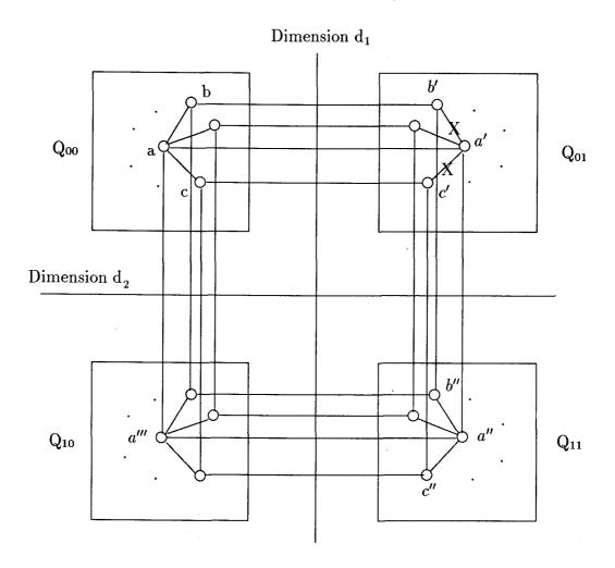
Figure 4.7. Case when all faulty links are incident to a single node. Link with X indicates faulty. Here node a' has two faulty links incident to it.
