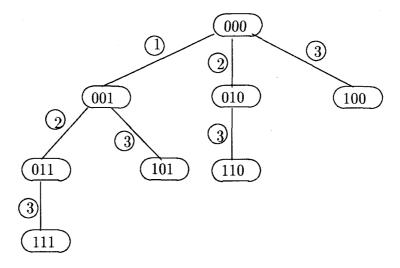
Figure 1.3. Broadcasting tree in  $Q_3$ . Here node 000 is a source node in  $Q_3$ .
