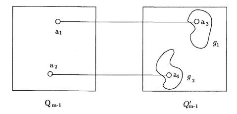
Figure 3.3. Division of  $Q_m$  into two subcubes. Every node in  $Q_{m-1}$  has broadcast message, and they are sending the message to corresponding nodes in  $Q'_{m-1}$ . Here some of the links connecting two subcubes may be faulty.  $g_1$  and  $g_2$  denote the sets of nodes disconnected in  $Q'_{m-1}$ . contains at least m-1 fewer faults than  $Q_m$ , and 3) is connected.
