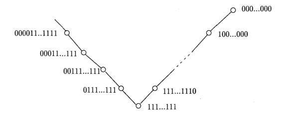
Figure 3.6. Generation of the longest possible fault diameter. Here m is the dimension of the cube and the number of faulty links allowed in  $Q_m$  is  $\frac{m^2}{2} - m - 1$ . Among all the links incident to nodes 111...111, 0111...111, 00111...111, 000111...111, ..., those links which are not shown in the figure are faulty.
