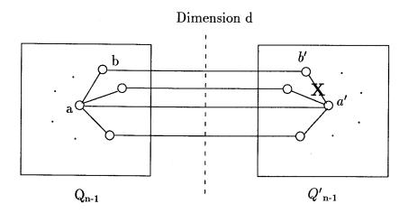
Figure 4.1.  $Q_n$  with one faulty link. Link connecting nodes a' and b' is faulty. the maximum number of faulty links incident to a node is f.
