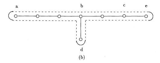
Figure 5.4. Two linear arrays formed by a HC with two faulty links. (a) Two linear arrays which result from the HC with two faulty links (a, g) and (f, k). Link (c, i) is not part of the HC and is called a bridging link. (b) Two linear arrays which result from the HC with two faulty links (a, d) and (e, d). In this case one linear array contains only one node. Link (b, d) is a bridging link.
