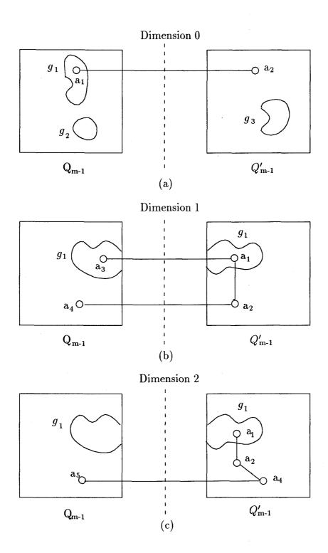
Figure 3.2. Division of  $Q_m$  along several dimensions.  $g_1$  through  $g_3$  denote the sets of nodes disconnected in the subcubes they belong.
