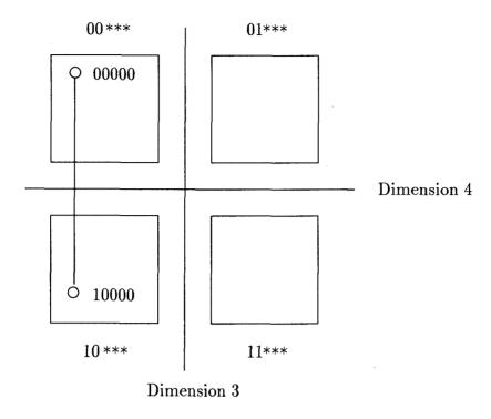
Figure 3.1. Division of  $Q_5$  along two dimensions.  $Q_5$  is divided first along dimension 3 and then along dimension 4. Node 00000 is the source node, and 0011-, 001-0, 00-00, 1100- are the faulty links.
