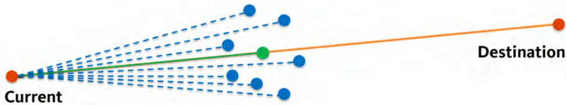
Figure 13: A visualization showing the candidate points and vectors (blue, dashed lines) which are compared to the target vector (green solid line) in Stage 2.
