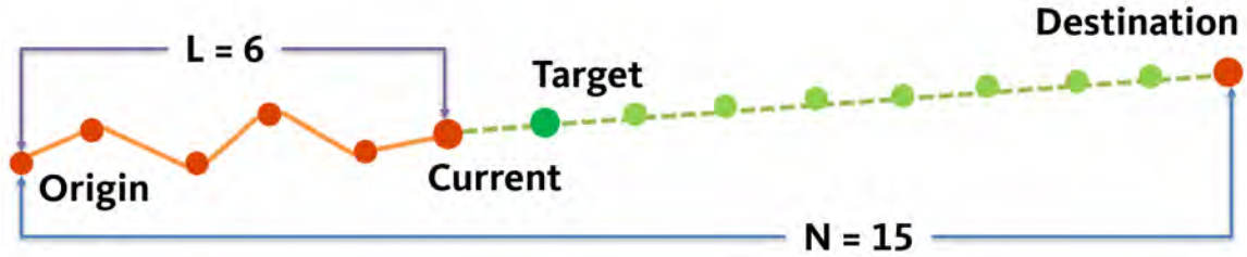
Figure 12: A diagram showing the target point in Stage 1 as the first step in a linear trajectory from the current point in the playlist to the destination.
