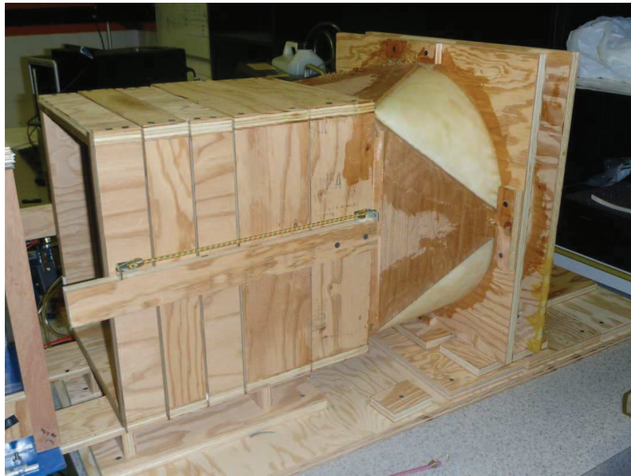
Figure 4-4: Blower with Flow Straightening Section
