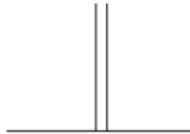
Figure 14: Geometry of sharp notch impinging interface used in cohesive modeling analysis.
