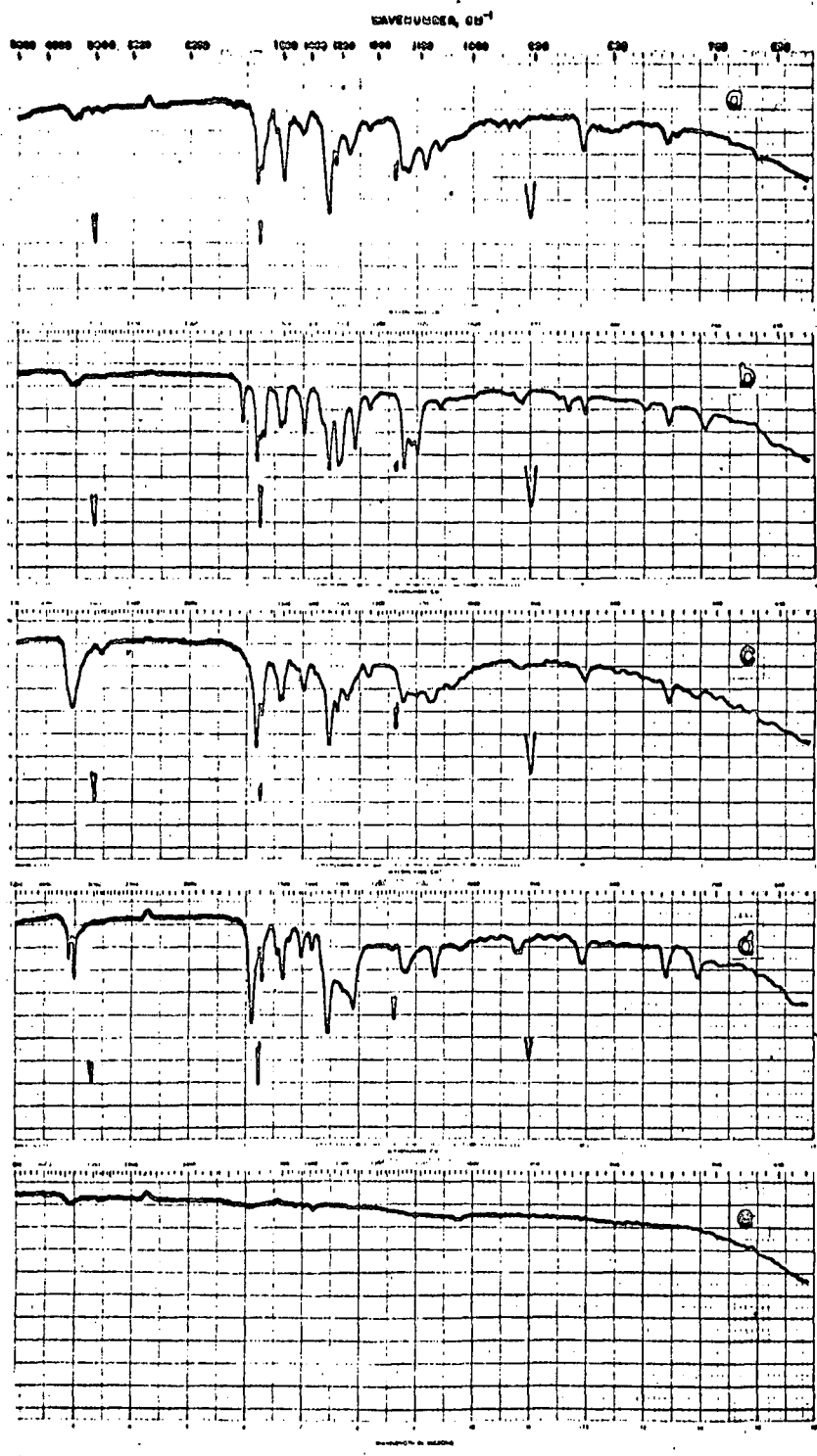
Figure 20. Infrared spectra of (a) diacetyl bis-(DNP-hydrazone), (b) diacetyl DNP-hydrazone, (c) acetoin DNP-hydrazone, (d) 2,4-dinitroaniline, (e) blank KBr pellet.
