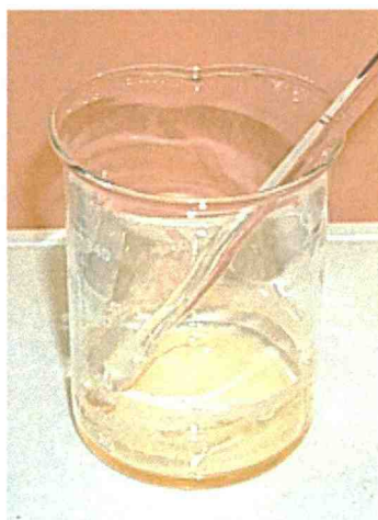
Figure 5: molten wax was being mixed with nifedipine
