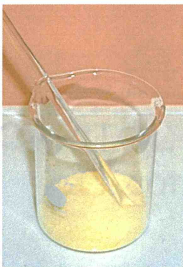
Figure 6: Sugar beads being coated by the mixture of wax and nifedipine
