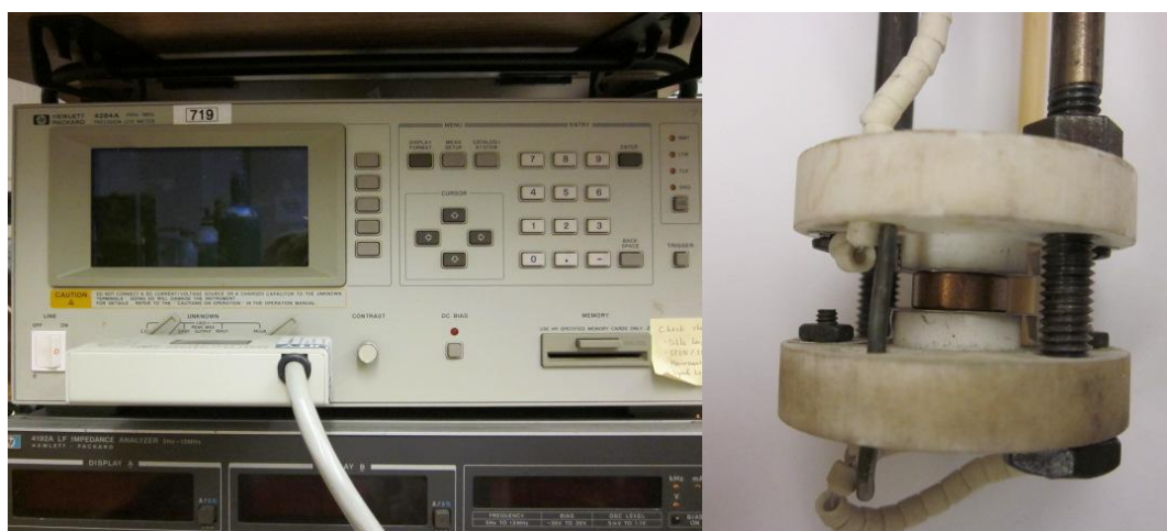
Figure 3.10: Dielectric set up with LCR meter (left) and two parallel electrodes (right).
