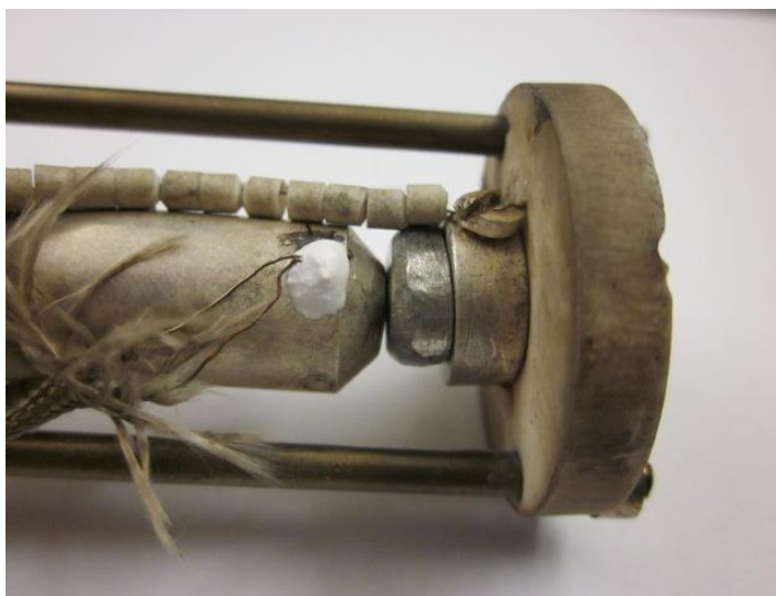
Figure 3.7: Set up for Seebeck coefficient measurement. Sample pellet is put in between two silver electrodes.
