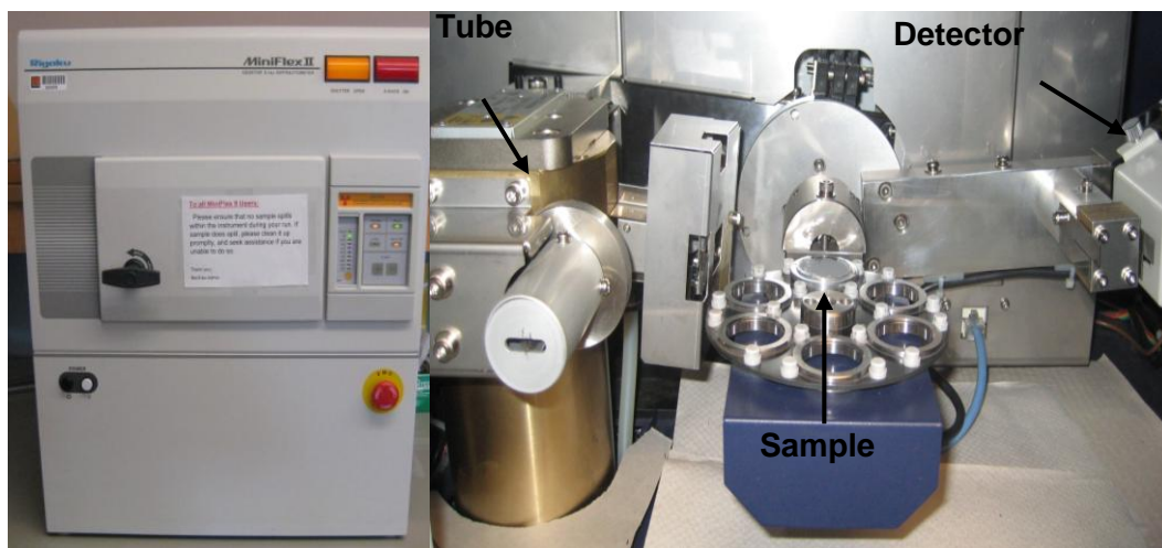
Figure 3.3: Rigaku MiniFlex II diffractometer (left) and the inner workings with X-ray tube, sample platform and detector labeled (right).
