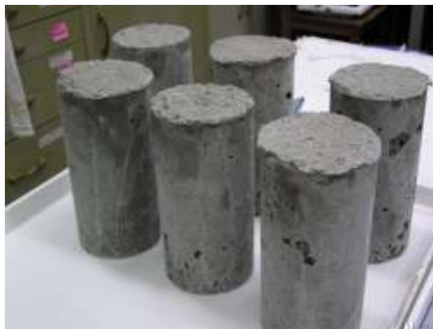
Figure 4.5 New Concrete Prior to Cut
