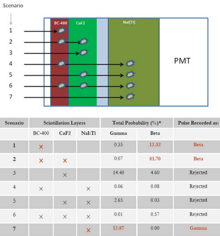
Fig. 2.2. The possible interaction scenarios in the triple-layer phoswich detector.
