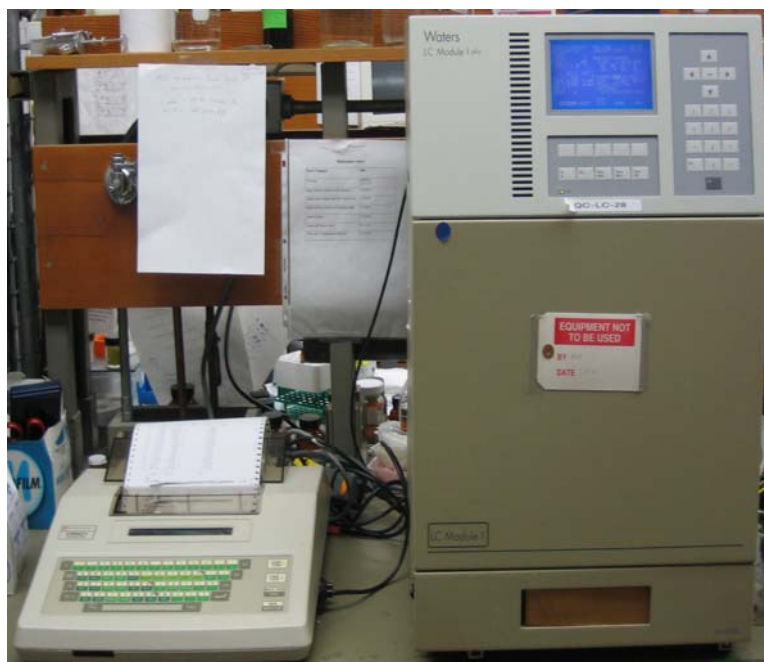
Figure 1.16. The HPLC machine, LC Module I, from Waters used to assay hydrocortisone
