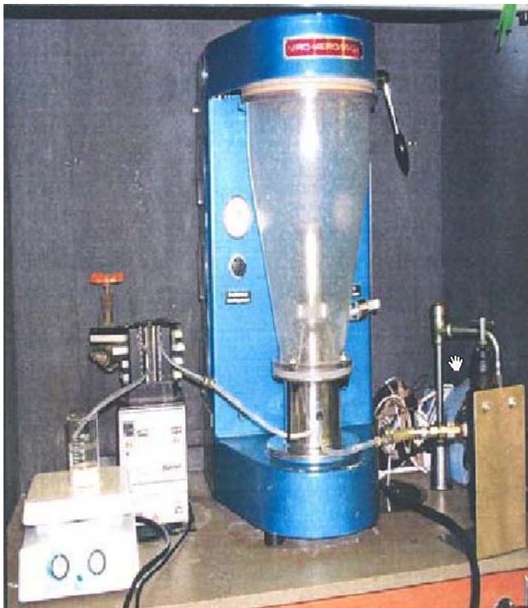
Figure 2.9. Spray coater used in the coating process, a fluid bed spray coater
