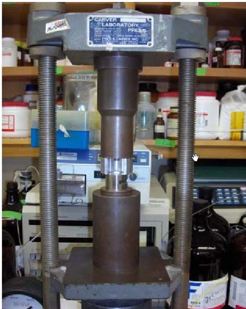
Figure 2.11. A simple tablet compressor used to make tablets
