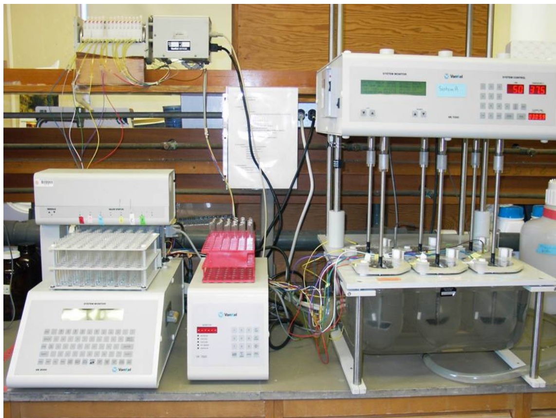
Figure 2.17. Dissolution machine, apparatus 2, to conduct dissolution studies on melatonin and acetaminophen tablets
