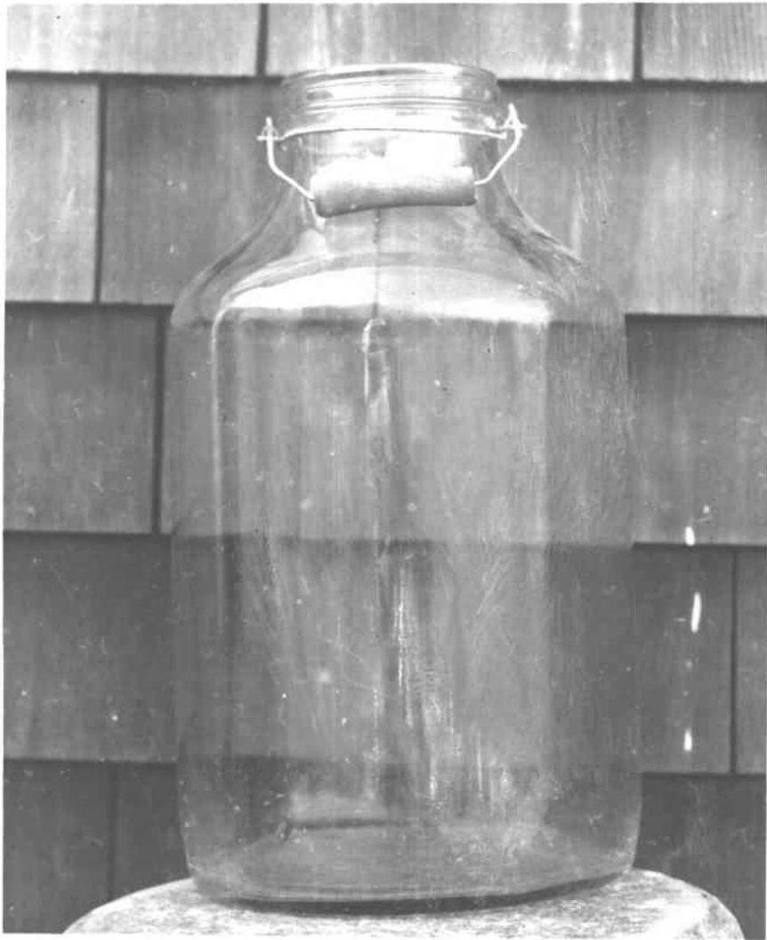
Figure 3. Five-gallon wide-mouth jars used in oyster larvae swarming and holding procedures.
