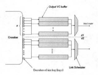
FIGURE 5.6: Modified Router Architecture
