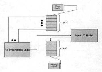
FIGURE 4.1: Flit Preemption Unit. This block is repeated for each input dimension in the Interconnect
