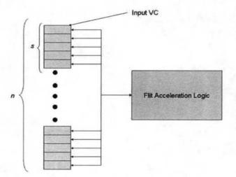
FIGURE 4.2: flit acceleration unit
