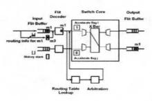
FIGURE 3.1: A higher priority message (m3) is blocked and needs to preempt a lower priority message (m1) in the input buffer using the extra buffer
