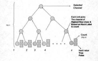
FIGURE 5.4: Hardware implementing the Modified Highest Non N-ACK Scheduling
