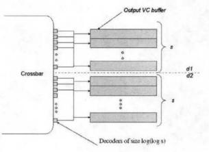
FIGURE 5.5: Flexible channel allocation at the Output VC Buffer
