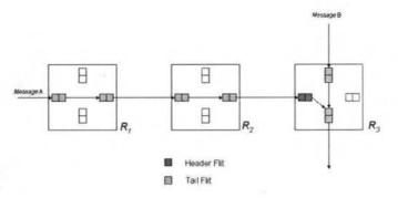
FIGURE 2.2: An example of blocked wormhole-switched message.
