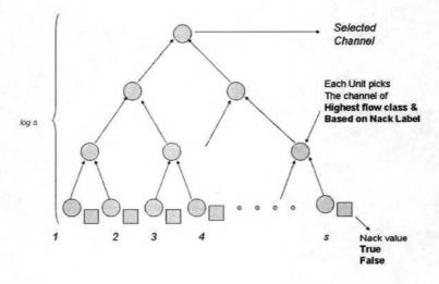
FIGURE 5.3: Hardware implementing Highest Non N-ACK Scheduling
