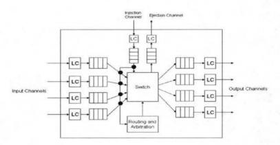
FIGURE 2.3: Generic router model.(LC = Link Controller)
