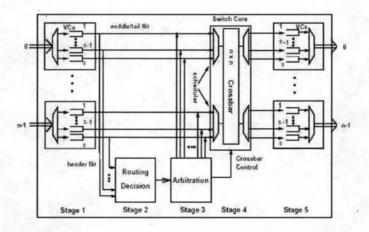
FIGURE 2.4: A five-stage pipelined router model
