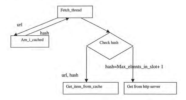
Get\_item-from\_cache module would call the get\_index module to get the hash\_index. The parameter hash would have the index into the linked list where the content is. With both these information the module retrieves the contents and returns it to the fetch\_thread. Now the module
