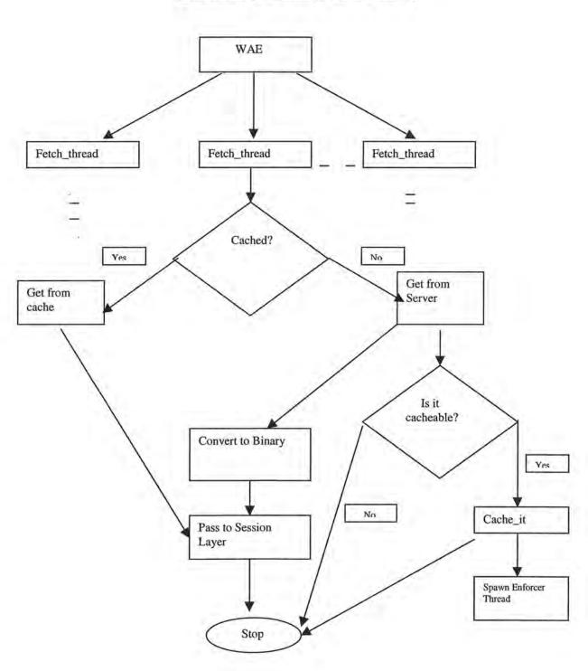
All the fetch\_threads being spawned and also the enforcers being spawned may access the cache simultaneously. Protecting the cache by a lock becomes necessary.
