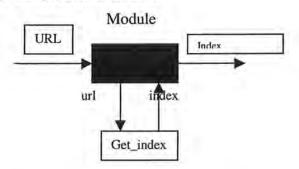
The fetch thread before doing the http server "get" would call the am\_I\_cached module with the specific url. The module would do the following steps.
