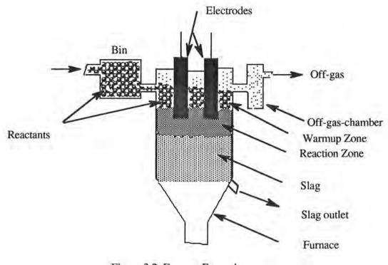
Figure 3.2: Furnace Example
