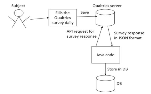
Figure 15. Interaction of the WavePipe Survey Reporter with Qualtrics server through its
