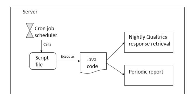
Figure 16. Functioning of a Cron job scheduler in the server
