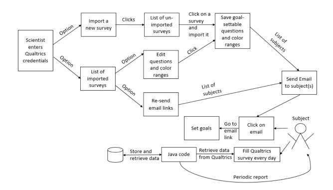
Figure 1. Use case covering the WavePipe Survey Reporter
