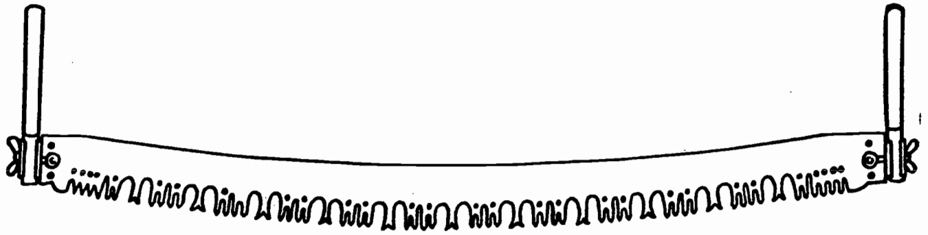
Two-man Racker-toothed Cross-cut-Saw
