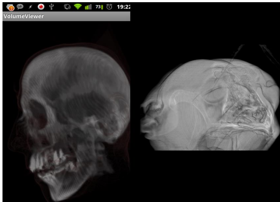
Figure 33 Left - The same example from Rodriguez as shown in the previous figure (Rodriguez, 2012) Right - Our implementation showing a sub-volume of the dog dataset. Notice how much more detail is in the image due to visualizing a subset of the native resolution dataset.
