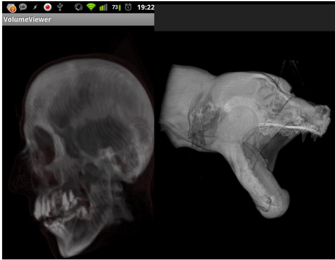
Figure 32 Left - Example of Rodriguez's implementation, a 256 x 256 x 113 skull dataset with 128 slices (Rodriguez, 2012) Right - Our own implementation at 500 steps.
