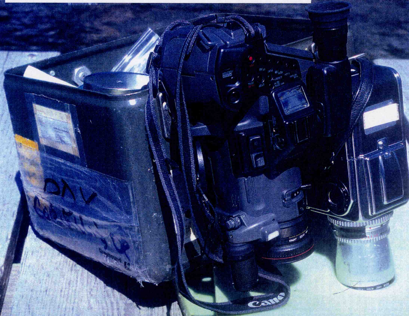
Figure 5: The camera set-up is compact, versatile, and cost efficient. The Canon A1 Hi8 digital video camera, left, can be controlled remotely and is monitored with an external monitor (not shown). The Hasselblad 70mm camera is used to collect high resolution panchromatic images of areas of geomorphic interest.
